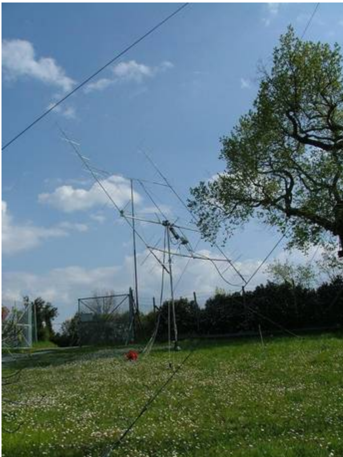
EME system 2x22XP DK7ZB, cavity preamp 0.4dB NF
